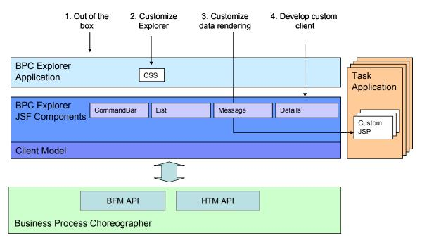
Figure 21: Structure of Business Process Choreographer Explorer and alternative uses
